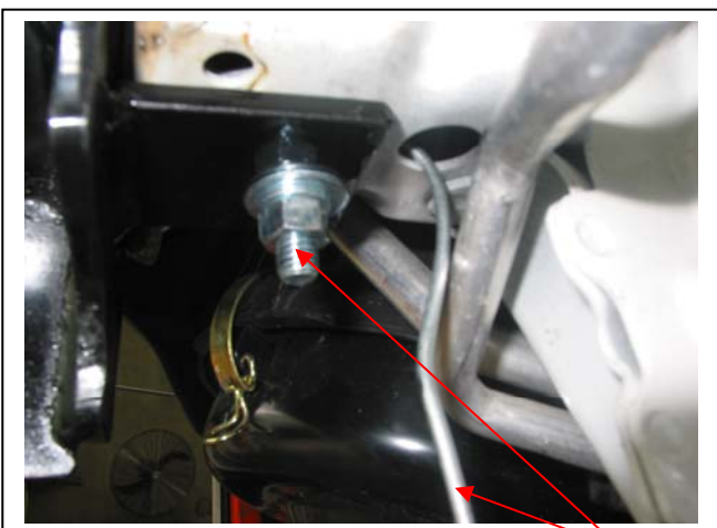
Figure 11 – Driver's side shown 3/8 x 1 1/4 bolt/wire
