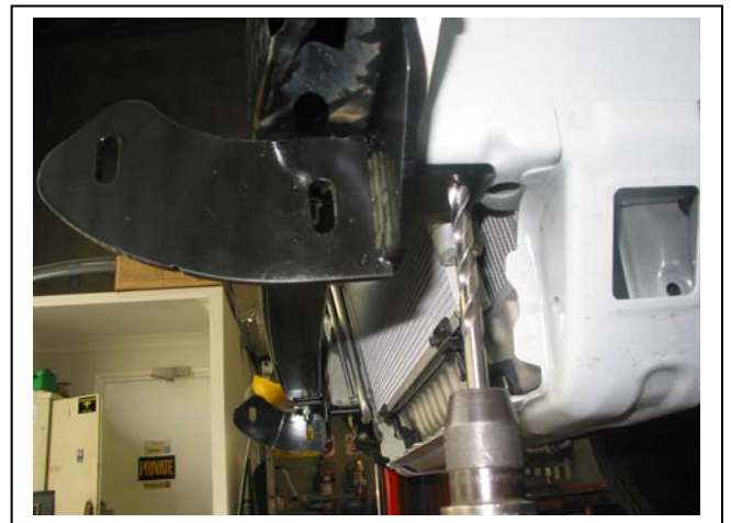
Figure 10 – Shown drilling passenger side chassis
