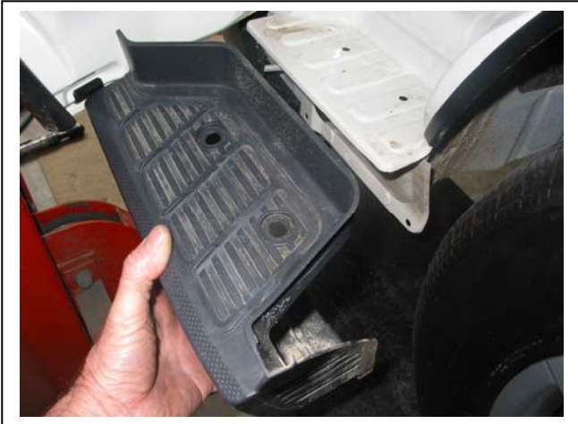
Figure 1 – Shown removing passenger side step infill
